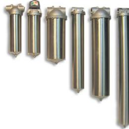
**SH and SHJ Series stainless steel single element housings** for DOE elements are robust and extremely affordable. They are available in 304 and 316 sst. SH series is for 2.5 inch diameter and SHJ is for 4.5" inch diameter filters. 3/4"- 1.5 NPT fittings available. *Conform to NSF/ANSI Std. 42*
