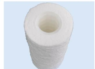
**DMC Series** melt blown polypropylene depth filters have a rigid molded internal polypropylene core to provide added strength where high-viscosity fluids or elevated temperatures could risk collapse of a coreless filter. *NSF/ANSI 61 available.*
