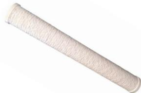
**RFC Series radial flow** cartridges have upstream and downstream melt blown polypropylene depth filter layers and activated carbon or other adsorptive medium packed inside. Grade PC plating carbon is great for electroplating bath cleanup.
