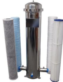
**FF Series** Filtration Systems consist of a rugged top-loaded stainless steel housings and 4.5" diameter x 30" length high capacity filter cartridges- a simple and economical system for filtration of water and various liquids up to 30 GPM.
