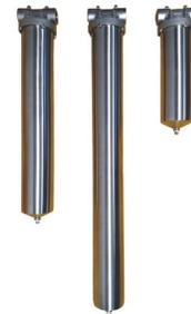
**SHU Series housings** of 304 and 316 stainless steel are single-element "Universal Style" vessels that accept DOE, 222 O-ring (flat top), and 119/213 O-ring (flat top) elements. These housings are robust and very affordable. 3/4" -1" NPT inlet and outlet available.
