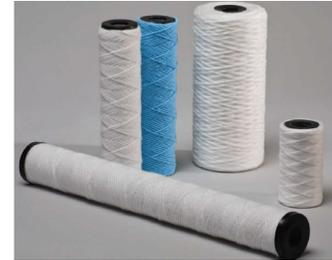
**CN04 and DCB Series Carbon/Sediment Filters** contain a wound section for pre-filtration and sediment removal, and a coconut shell based activated carbon section downstream for reduction of chlorine, bad tastes, and organics.
