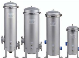
**BCV Series** Band Clamp Liquid Cartridge Filter Vessels have a heavy duty self-centering band clamp with O-Ring seal for convenient cartridge access and change out. Compatible with a wide range of fluids and hold various amounts of different sized cartridges.
